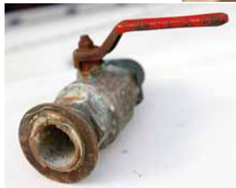
TOP: This cheap ball valve simply disintegrated with corrosion.
