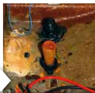
With the fitting smashed away completely, leaving a round hole, the bung forms a perfect seal
