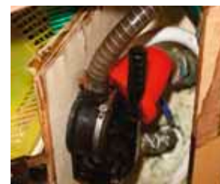
A perfect seal in the cracked tailpipe, but TruPlug is very big
