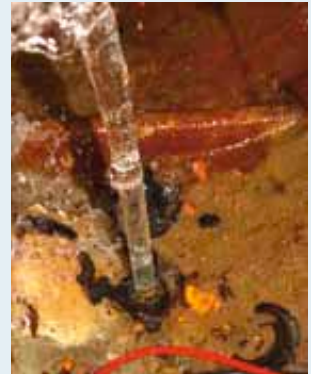
Next we smashed the fitting away at hull level, leaving a hole that gushed impressively
