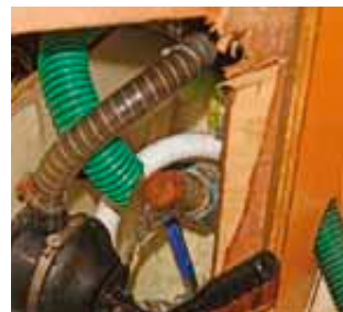
With a cracked tailpipe, the bung leaves a fairly serious leak
