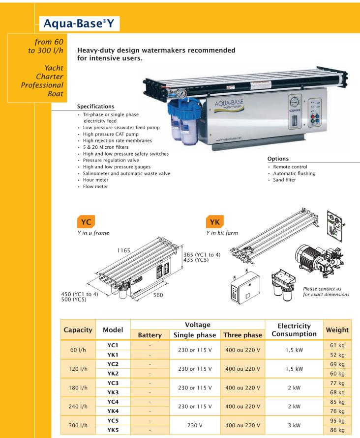
Rated performances +/- 10% using standard seawater, with 35 g/l salinity and temperature at 25°C. Other voltages on request.
