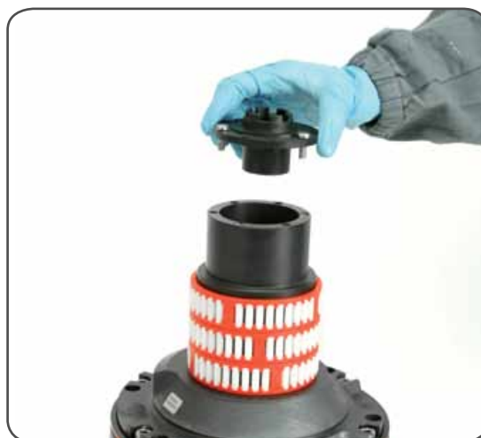
7. Remove the stripper arm housing n°21
