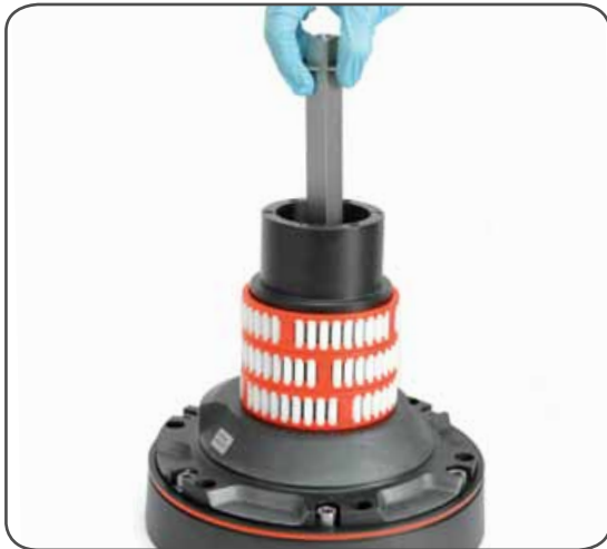
8. Slide out the central shaft n°19
