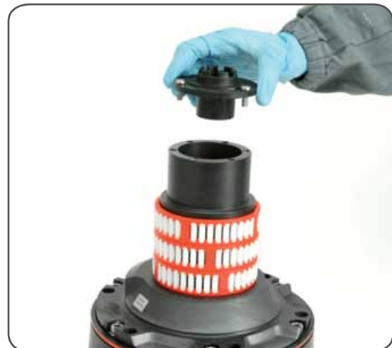
7. Remove the stripper arm housing n°21
