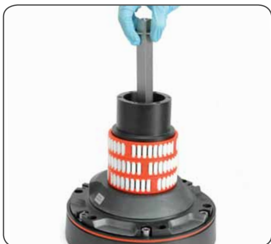
8. Slide out the central shaft n°19
