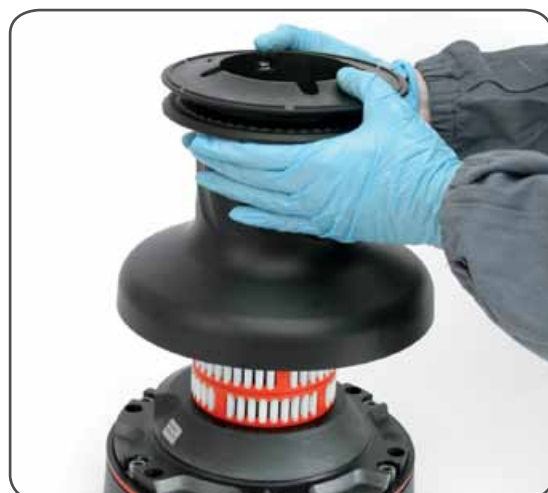
5. Lift off the drum n°24
