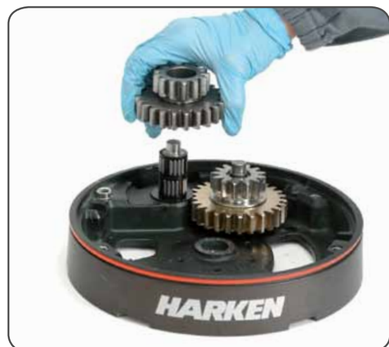
13. Remove the idler and pinion n°14
