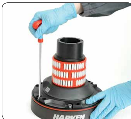
9. Unscrew the 6 hex screws n°17 ( \text{20Nm/177 in-lb} )
